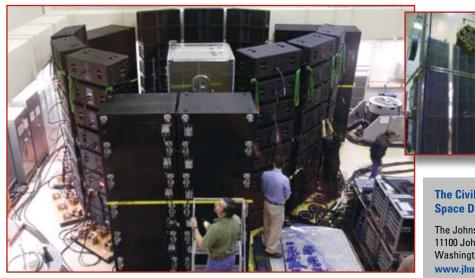
Acoustic tests for Radiation Belt Storm Probes provided an opportunity to test Solar Probe materials with an acoustic blast.
